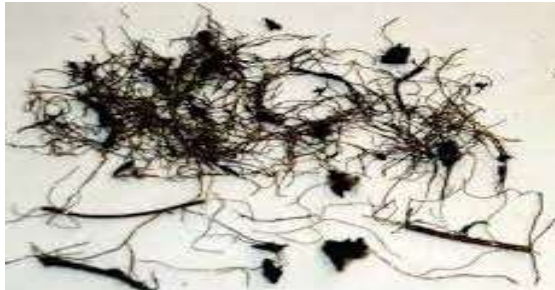
FIG 3.2 RECYCLED TYRE STEEL FIBRE
